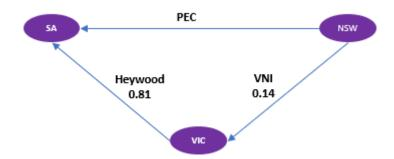
AEMO intends to reflect PEC in the network model for dispatch. This will create a parallel transmission configuration between the regional nodes of South Australia, Victoria and New South Wales.
